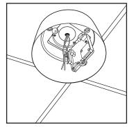
NOTE: If installing outdoors apply a sealant between the back box and the mounting surface
